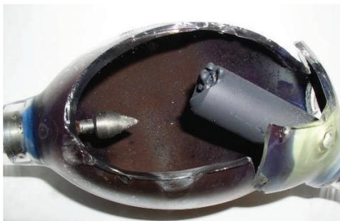
A gradual and even blackening of the lamp envelope, and the reduced output of light usually indicates a slow seal failure.
