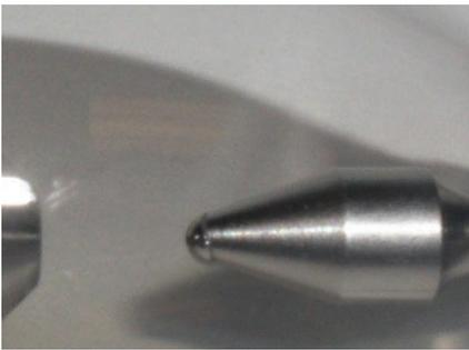
**ANODE:** The larger electrode suffers the brunt of the Electrode related problems, as it is on the receiving end of the arc flame. Proper evaluation of the damage can typically identify the problem, or at least simplify the analysis. When excessive ripple is present in the DC input, the result will be
