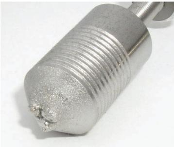
Incorrect current outside the lamp's rating will also damage the anode by the flame literally blasting the anode material away, or leaving deposits due to incorrect operating temperature.
