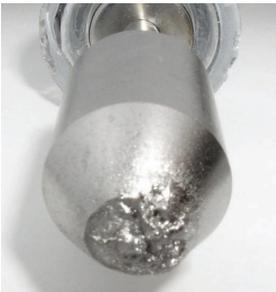
Lamp position and/or incorrect magnetic stabilization will also affect the lamp. If the lamp is operated at an excessive angle, the flame will drift away from the center of the anode, and leave deposits that will lead to flicker. In the same principle, if there is missing or incorrect magnetic stabilization, the flame will react in the same manner, drifting away from the center and leaving deposits that will permanently cause flame instability.
