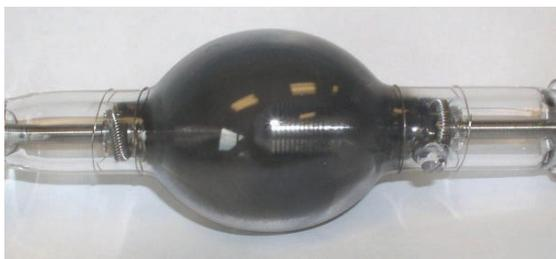
Re-check the cooling system to make sure the airflow is proper, unrestricted, and directed properly. Over-heating of the lamp is the primary cause of seal failures. In addition, make sure the method of mounting the lamp does not induce physical stress on the lamp
