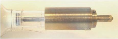
While excessive overheating will turn the end caps black, and cause the seal underneath to fail. In extreme cases, the danger of explosion is present.
