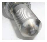
Dis-Colored End Fittings are the result of improper cooling / lamp overheating, or in rare cases, the reflector focusing the light on the lamp end. Mild over-heating will turn the fittings a blue color.
