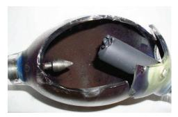
A gradual and even blackening of the lamp envelope, and the reduced output of light usually indicates a slow seal failure.
