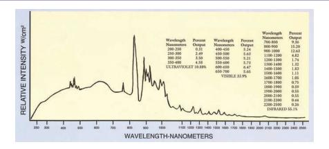
The white color output of xenon lamps makes them a perfect fit for film and image projection applications. In addition, xenon lamps are also used in solar and space simulators, search and spot-lights, and other specialized lighting applications needing a bright white light source.
