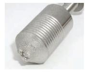
Incorrect current outside the lamp's rating will also damage the anode by the flame literally blasting the anode material away, or leaving deposits due to incorrect operating temperature.
