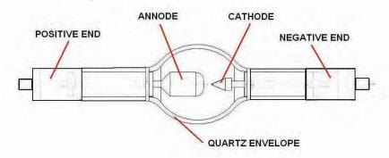
A Xenon Lamp is comprised of a simple construction in theory, yet the assemblies and parts are all highly specialized. The diagram below shows the basic layout only, hiding many of the details. Listed below is a simplified overview of a typical Xenon lamp:
