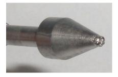
Reversed polarity of the DC connections will also quickly cause a melted cathode
