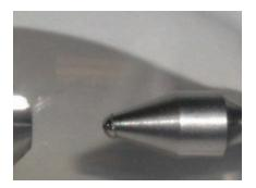
ANODE: The larger electrode suffers the brunt of the Electrode related problems, as it is on the receiving end of the arc flame. Proper evaluation of the damage can typically identify the problem, or at least simplify the analysis.
